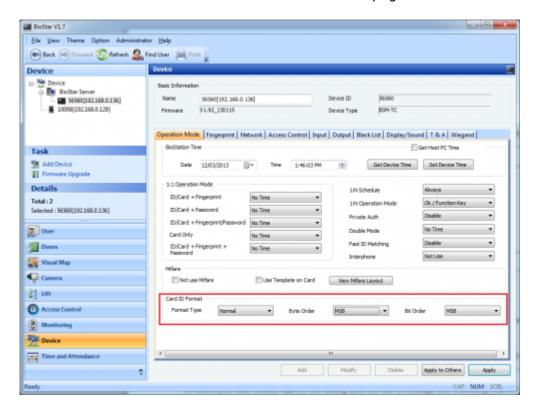
How do the settings of the byte and bit orders affect card reading?
