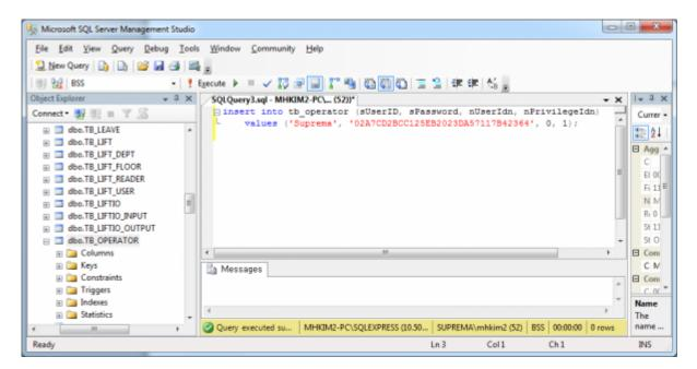
1) Type the following query in the query editor: insert into tb\_operator (sUserID, sPassword, nUserIdn, nPrivilegeIdn) values ('Suprema', '02A7CD2BCC125EB2023DA57117B42364', 0, 1);
