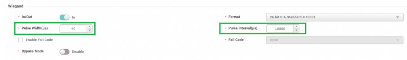
3. Since the suprema device is sending the signal out to the controller, the Wiegand signal should be set to \*Out\*.
