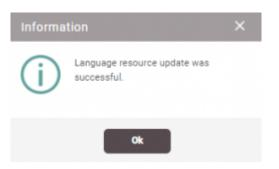
9. The device will reset after applying the resource file. Go back to the **Display/Sound** settings and change the **Language** to **Custom**. Press **Apply**.
