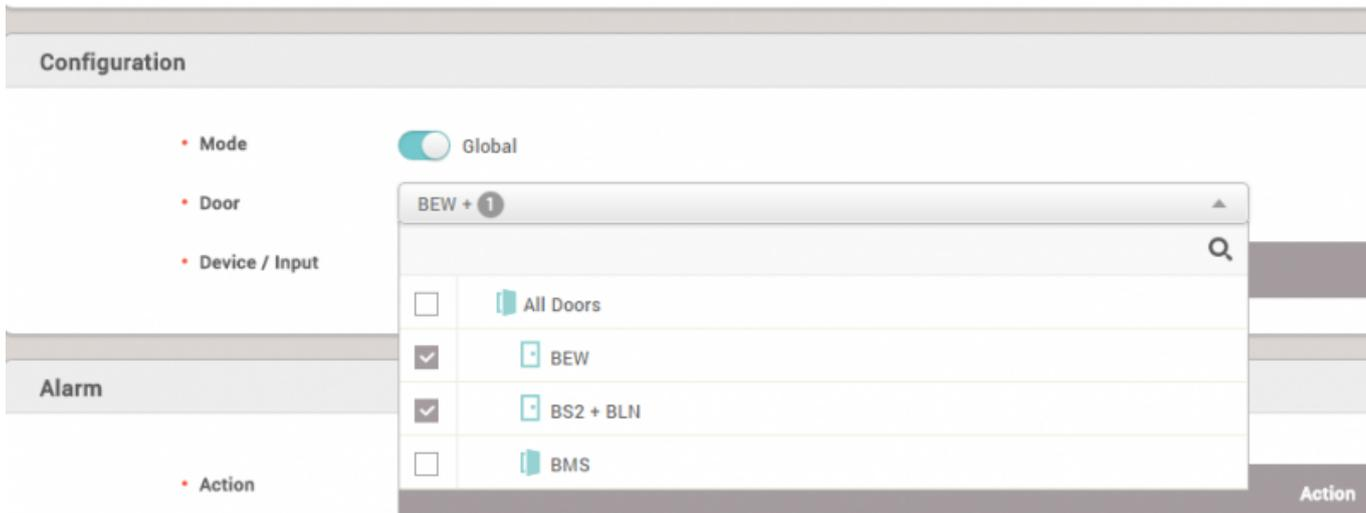
3. Choose the doors that will be in the fire alarm zone and select a device input to receive fire alarm signals.
