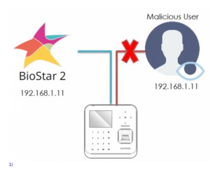
This security option is achieved by storing a digital certificate in the device. When the device connects to the server, it will exchange an encryption key (session key) using the digital certificate to provide server identity verification.
