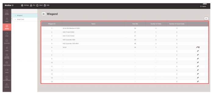
3. Wiegand format can be set by assigning the total bits, ID field, and parity bits. For example, in order to configure 34 bits card format with parity bit checks by half of each even and odd parity check logic, it's necessary to set 'Start Bit' and 'End Bit' for each part.
