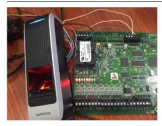
8. Check 3rd party system monitoring, and input value. If there are no events and responses, check the wiring and pulse and Wiegand format. If there are error message, please try to change the card ID format and reading mode, such as **Byte Order**.
