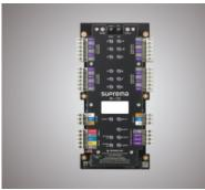
Input Module is a multiple input extension module which can control up to 12 supervised inputs, 2 AUX, 1 temper switch and 2 relays. A total of 31 units can be connected to a master device via an RS485 daisy chain. It allows the use of inputs for interfacing with sensors or door contacts etc., as well as providing a simple 'dry contact' interface for other systems.
