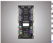
Input Module is a multiple input extension module which can control up to 12 supervised inputs, 2 AUX, 1 temper switch and 2 relays. A total of 31 units can be connected to a master device via an RS485 daisy chain. It allows the use of inputs for interfacing with sensors or door contacts etc., as well as providing a simple 'dry contact' interface for other systems.
