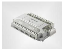
Door Module provides secure door control of up to four doors via encrypted communication and also contains two Wiegand reader interfaces for use with 3rd party readers. A wide variety of I/O interfaces allows Door Module to be a part of diverse system configurations.
