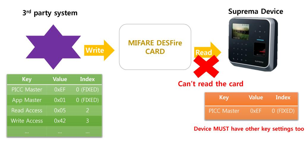
DESFire advanced option allows Suprema device to read card issued by 3<sup>rd</sup> party system even with different key setting
